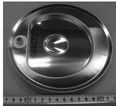
写真 9 絞り、穴広げ加工品の例 Photo 9 Example of stamped part by drawing and expanding
