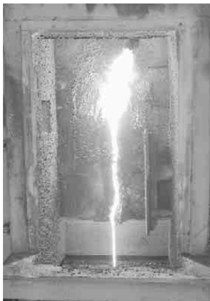
Photo 1 Continuous tapping of molten slag
