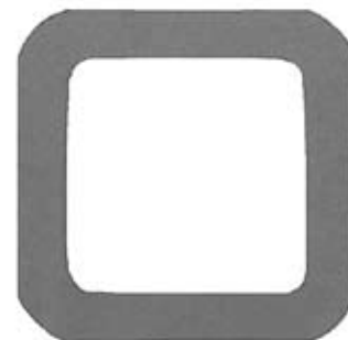
Fig. 3 Cross-sectional shape of JFE Kakuhot (Side length: 250 mm, Wall thickness: 36 mm)
