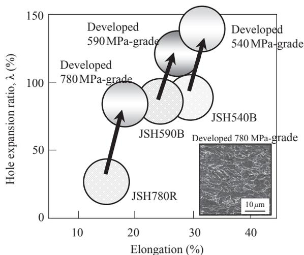
Fig. 1 Balance of elongation and hole-expansion ratio
