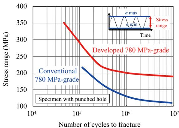
Fig. 2 Fatigue properties
