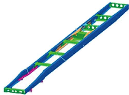
Fig. 4 Application of developed 780 MPa-grade steel to truck frame
