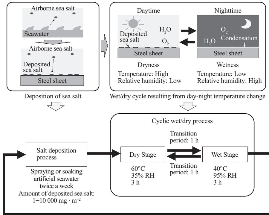
Fig. 4 Example of test conditions of new accelerated corrosion test "ACTE"<sup>24–28)</sup>
