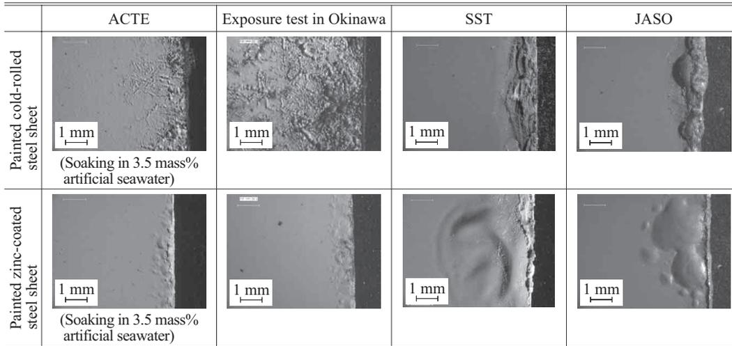
Photo 1 Comparison of corrosion morphology of painted steel sheets
