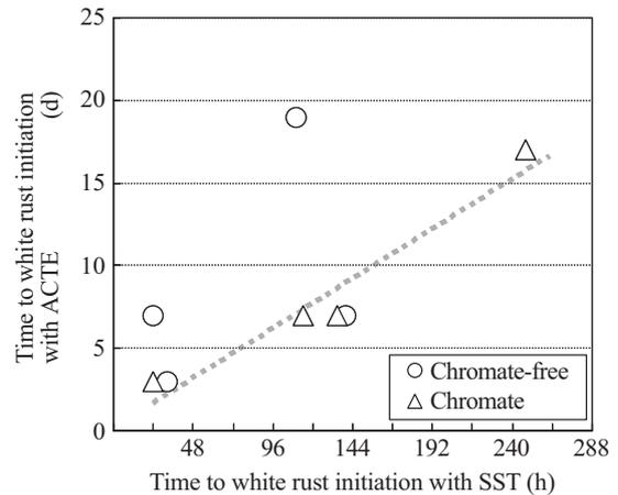
Fig. 7 Comparison of time to white rust initiation with ACTE and SST<sup>24)</sup>
