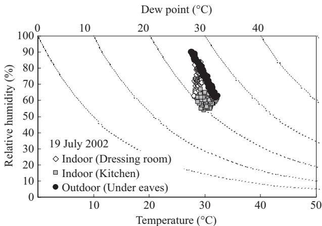
Fig.3 Relationship between temperature and relative humidity in actual environment where electrical appliances were used
