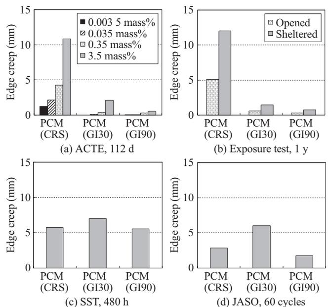
Fig.6 Comparison of corrosion from edges of painted steel sheets<sup>27)</sup>
