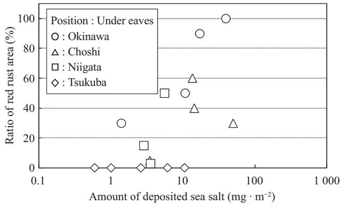
Fig.2 Relationship between amount of deposited sea salt and corrosion of collected air-conditioners (air vent of side cover)<sup>23,25)</sup>
