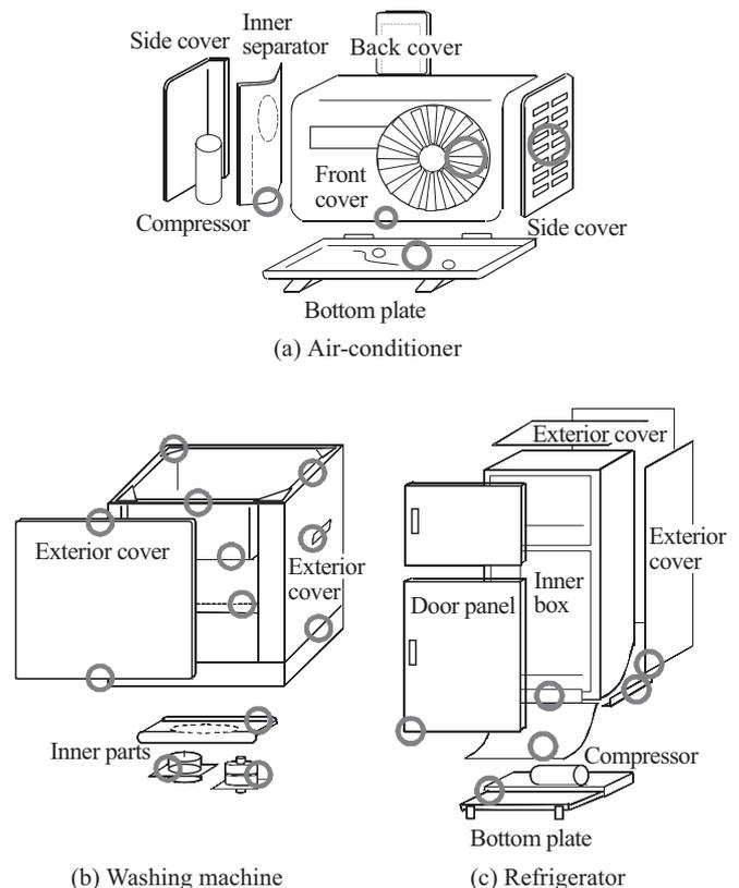
Fig. 1 Location of parts of electrical appliances with high susceptibility to corrosion<sup>19,20)</sup>
