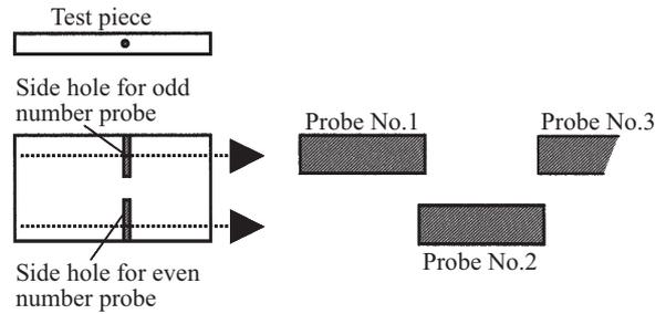
Fig. 9 Test piece and scanning method over probes
