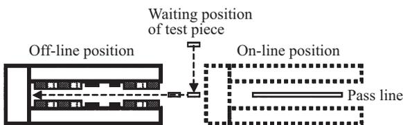
Fig. 7 Movement of test piece at sensitivity adjustment
