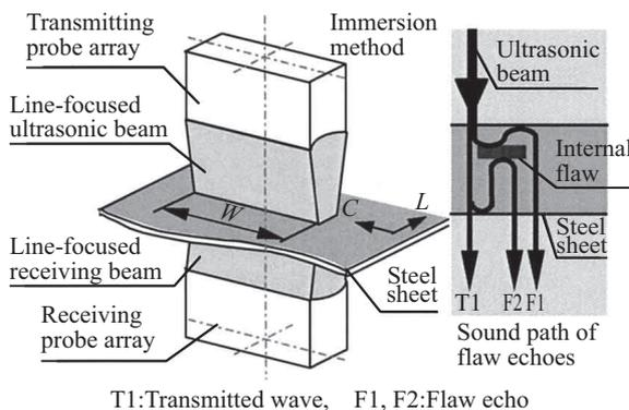
Fig.1 Schematic geometry of ultrasonic probes
