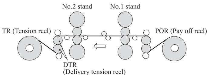
Fig.2 Fukuyama No. 3 TMP
