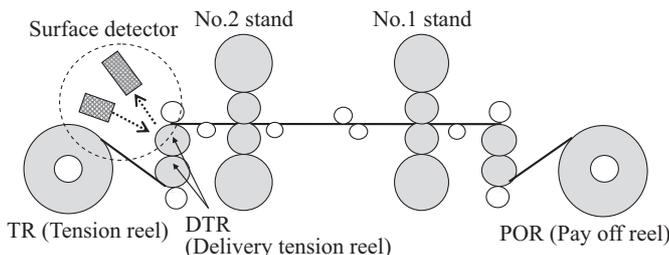
Fig. 5 Place of the “surface detector”
