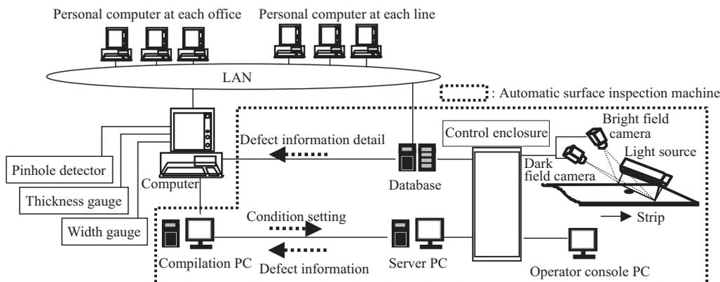
Fig.2 System configuration of automatic surface inspection machine
