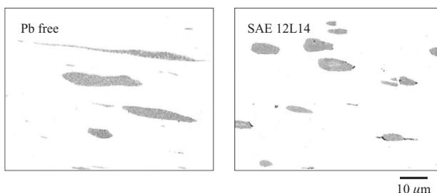
Photo 2 Size of sulfide inclusions of Pb free steel in comparison with SAE12L14 steel
