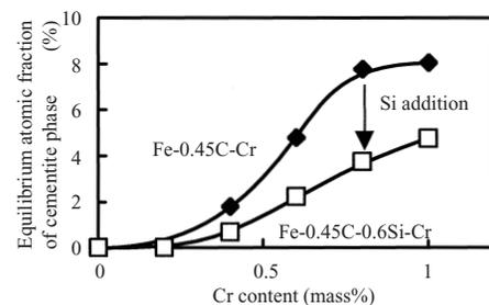
Fig. 2 Effects of Cr and Si on stability of cementite phase at 700°C
