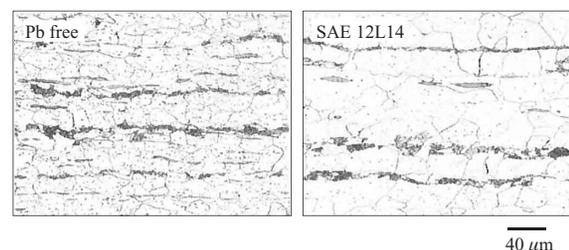
Photo 1 Micro structure of Pb free steel in comparison with SAE12L14 steel
