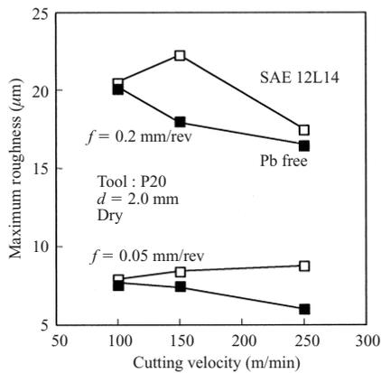
Fig. 9 Maximum roughness of Pb free steel in comparison with SAE12L14 steel
