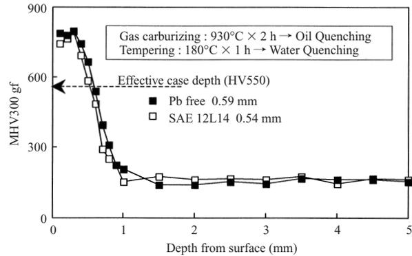
Fig. 11 Carburization characteristics of Pb free steel in comparison with SAE12L14 steel
