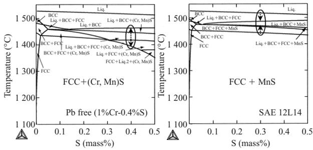
Fig. 5 Examples of calculated phase diagrams
