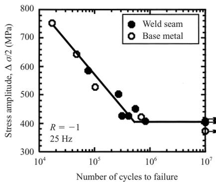
Fig.5 Fatigue endurance (S-N) curves of weld seam and base metal in 780 MPa ERW steel tube
