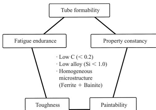
Fig.2 Concept of developed 780 MPa ERW steel tubes
