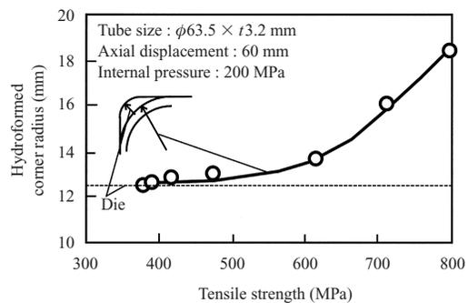
Fig. 7 Effect of tensile strength on hydroformed corner radius in die cavity
