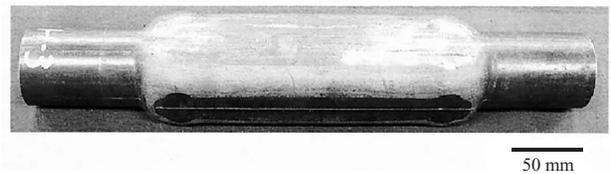
Photo 2 Hydroformed 780 MPa HISTORY in die cavity ( $\phi 63.5 \times t3.2$  mm  $\rightarrow$  35% expansion)
