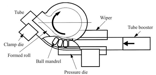
Fig.6 Schematic illustration of rotary draw bending
