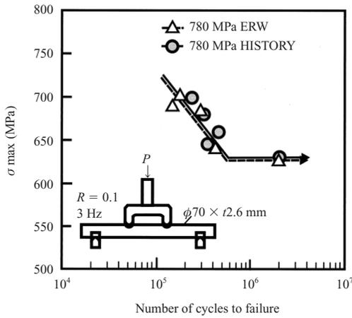
Fig.4 Fatigue endurance (S-N) curves of developed 780 MPa ERW steel tube and 780 MPa HISTORY in 4-point bending fatigue test
