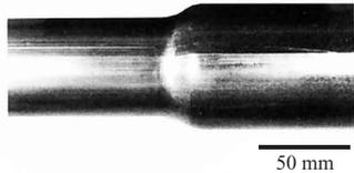
Photo 1 20% swaged 780 MPa ERW steel tube ( $\phi 76.3 \times t2.9 \rightarrow \phi 60.5$  mm; 1 pass)
