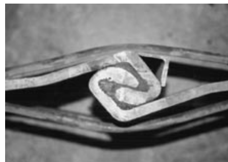
Photo 5 Steel sheet pile joints with polymer seals swelled with water
