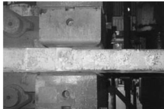
Photo 1 Forging reduction in thickness of CC slab
