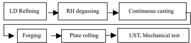
Fig.5 Manufacturing process
