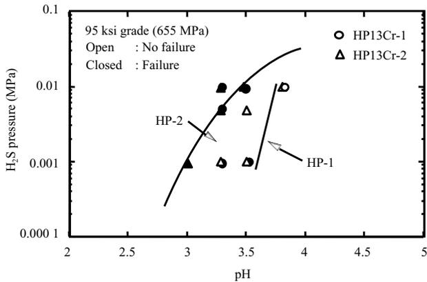
Fig. 17 SSC test result for HP13Cr pipe
