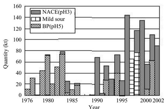
Fig. 10 Production amount of sour gas linepipes
