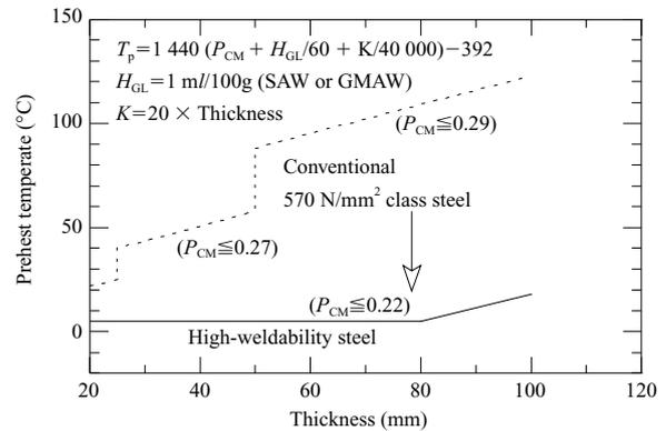
Fig.2 Example of the decrease in required pre-heat temperature for low  $P_{CM}$  HSLA steel plates<sup>2)</sup>
