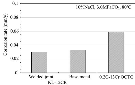
Fig. 18 CO<sub>2</sub> corrosion test results of KL-12CR welded joint
