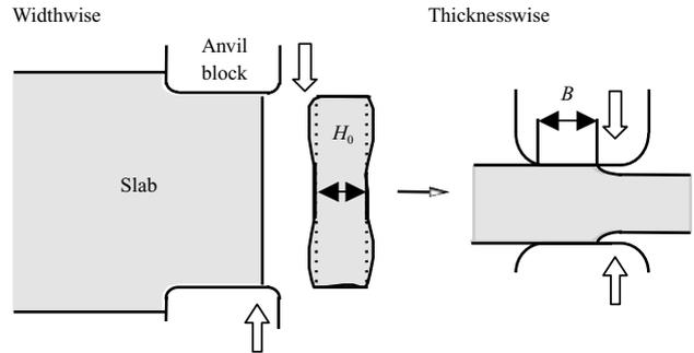
Fig.6 Schematic diagram of CC slab forging
