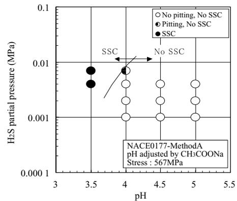
Fig. 19 SSC test results of KL-HP12CR welded joint
