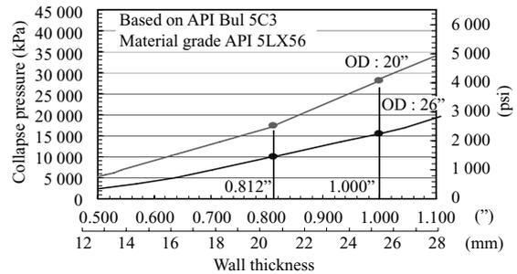
Fig. 14 Calculated maximum collapse pressure for heavy wall pipe
