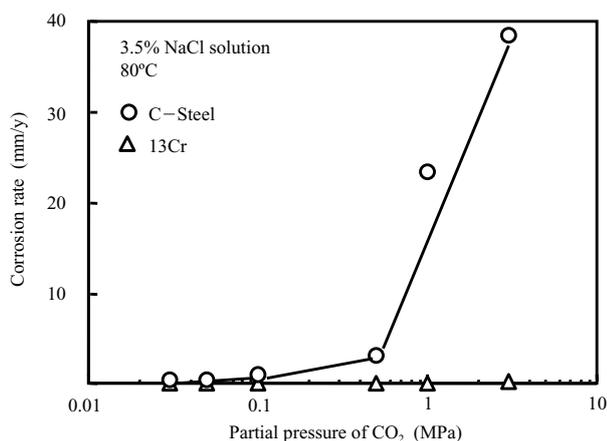
Fig. 15 CO<sub>2</sub> corrosion test result
