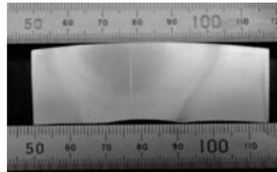
Photo 2 ERW weld seam of 1.000" thick pipe (Nital etched)
