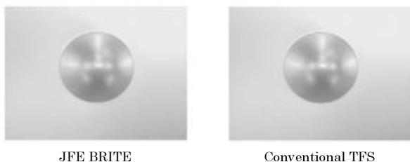
Photo 5 Results of humidity cabinet test (Temperature : 30°C, Humidity : 70–80%, 3d)
