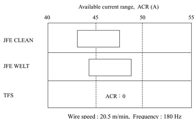
Fig. 11 Weldability of JFE CLEAN in comparison with JFE WELT and TFS
