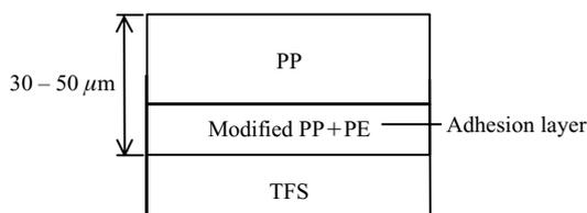
Fig. 6 Cross section of PP laminated steel sheet for 18 l can
