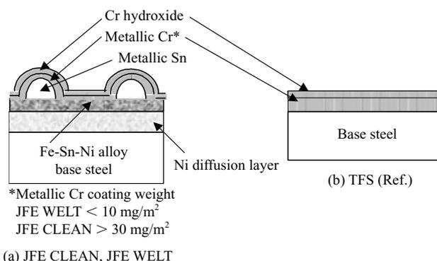
Fig. 10 Schematic cross-sectional views of JFE CLEAN, JFE WELT and TFS
