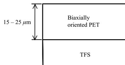
Fig. 8 PET laminated steel sheet for 18 l can
