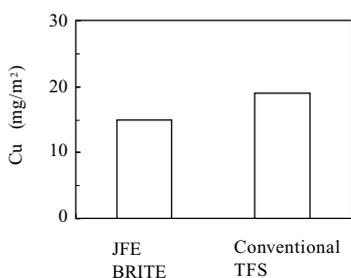
Fig.9 Cu extraction obtained by the CuSO<sub>4</sub> dipping test
