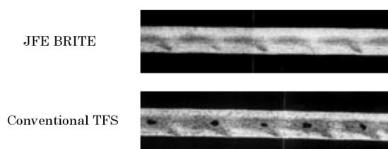
Photo 4 Longitudinal sections of the welds
