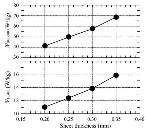
Fig. 8 Influence of sheet thickness on iron loss at high frequency
