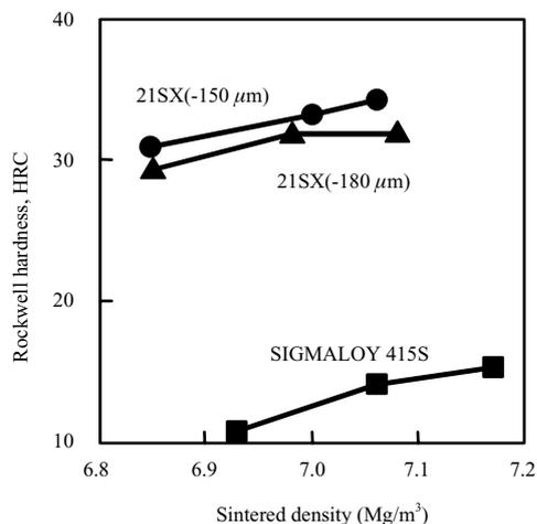
Fig. 17 Relations between sintered density and hardness of sintered compacts made of KIP 21SX and SIGMALOY 415S
