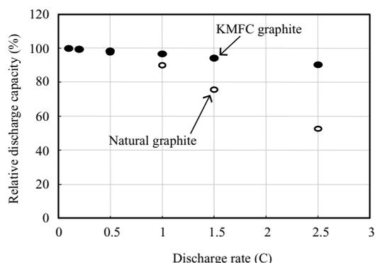
Fig. 19 Comparison in relative discharge capacity of developed KMFC graphite powders and natural graphite powders
