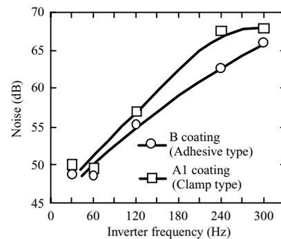
Fig. 10 Comparison of B and A1 coatings in noise emitted from model motor
