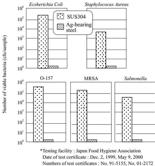
Fig. 13 Results of antibacterial test\* of 0.042 mass% Ag-bearing steel
