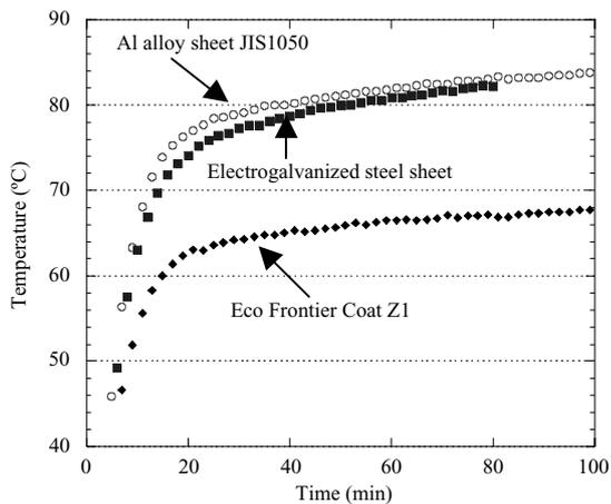
Fig. 1 Temperature increase inside a radiation tester
