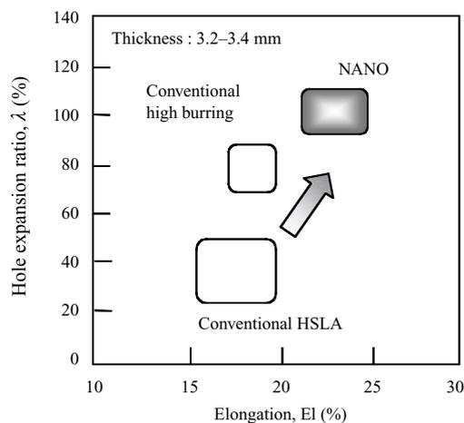
Fig. 1 Comparison of EI- $\lambda$  balance of 780 MPa grade hot rolled steels
