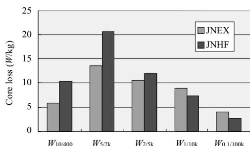
Fig. 20 Core loss comparison data between JNEX and JNHF
