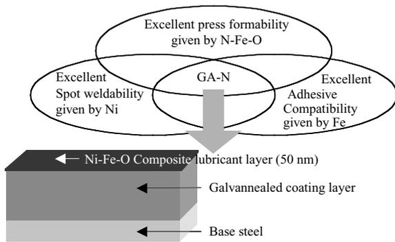
Fig.8 Basic concept and cross sectional view of GA-N
