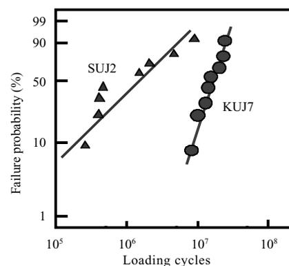
Fig.26 Rolling contact fatigue life at 180°C
