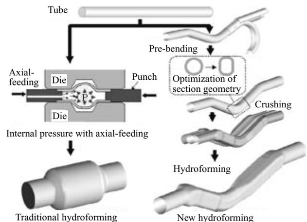
Fig. 14 Manufacturing process of hydroformed tube
