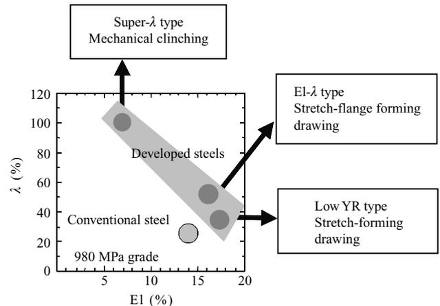
Fig.6 Typical EI- $\lambda$  balance of newly developed 980 MPa grade ultra-high strength steels
