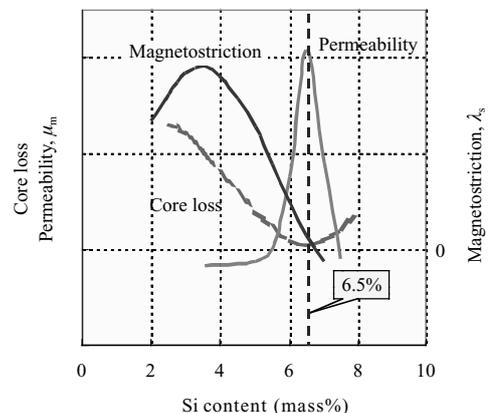
Fig. 19 Variation of magnetic characteristic by Si content of Fe-Si alloy
