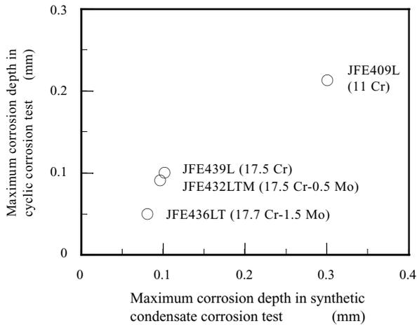
Fig.21 Comparison of corrosion resistance between steels for muffler
