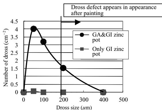
Fig.9 Number of dross on galvanized steel sheet
