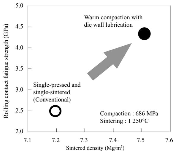
Fig. 30 Relation between sintered density and rolling contact fatigue strength of sintered and carburized steel compacts made of 2Ni-1Mo partially alloyed steel powder
