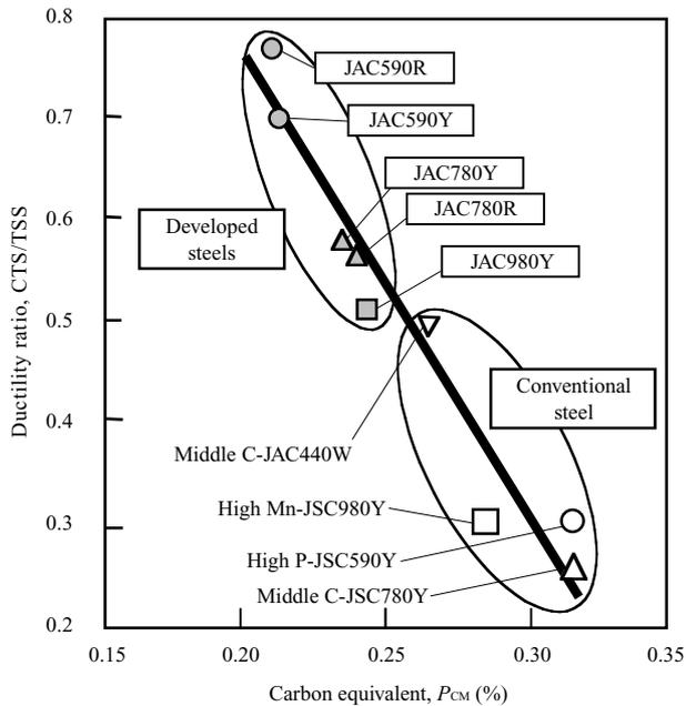
Fig.5 Relationship between ductility ratio, CTS/TSS and carbon equivalent,  $P_{CM}$  at welding current of 7.5 kA
