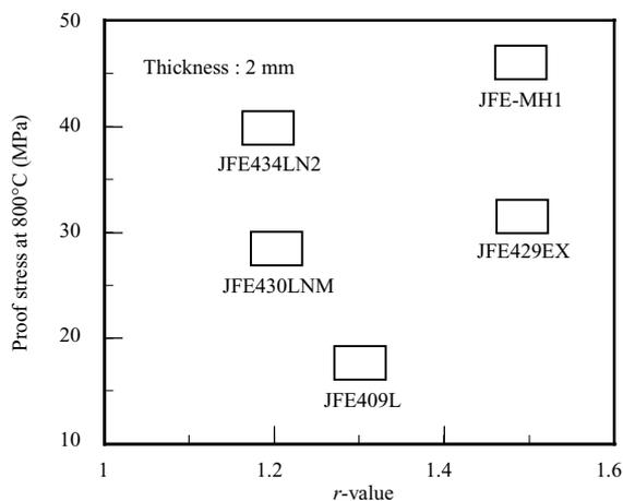
Fig.22 Comparison of  $r$ -value and PS at 800°C between steels for exhaust manifold
