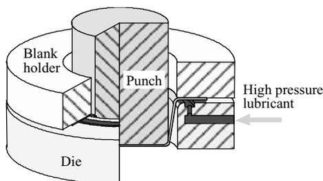
Fig. 15 High pressure liquid lubrication method
