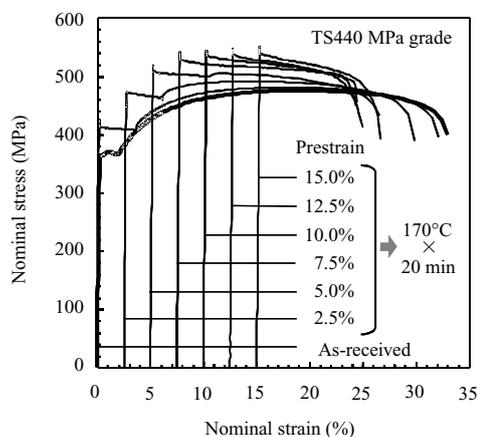
Fig. 2 Stress-strain relationship of newly developed steel after strain aging
