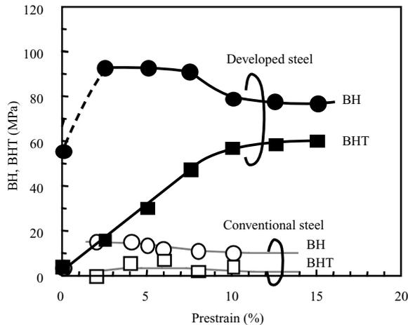
Fig.3 Effect of prestrain on BH and BHT of newly developed steel after strain aging ( $t = 1.4$  mm)
