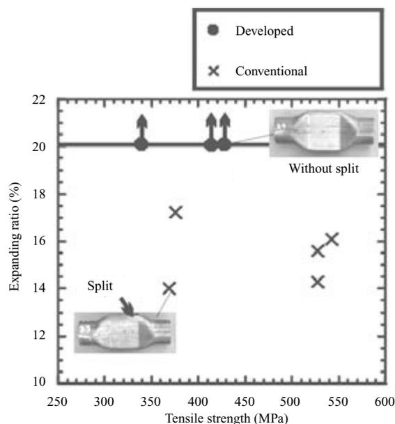
Fig. 25 Relationship between tensile strength and tube hydroformability of the developed and the conventional tubes in rectangular die cavity (Maximum expanding ratio = 20%)
