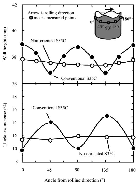
Fig. 7 Change in wall height and wall thickness after cup cylinder deep drawing
