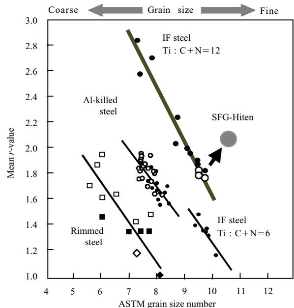
Fig.4 Correlation between mean  $r$ -value and grain size in both SFG-Hiten and other conventional steels
