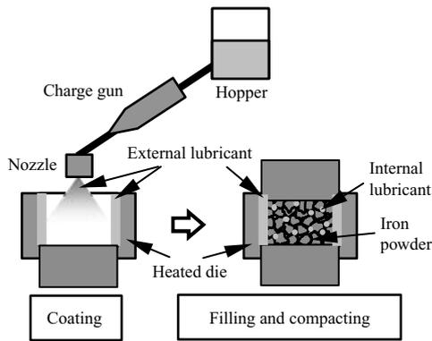
Fig. 29 Schematic diagram of warm compaction method with die wall lubrication
