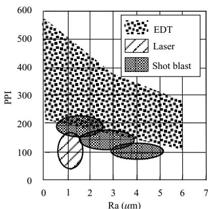
Fig. 10 Influence of skin-pass roll texturing technology on PPI and roughness
