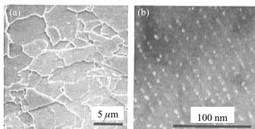
Photo 1 Microstructure (a) and precipitates (b) of NANO Hiten
