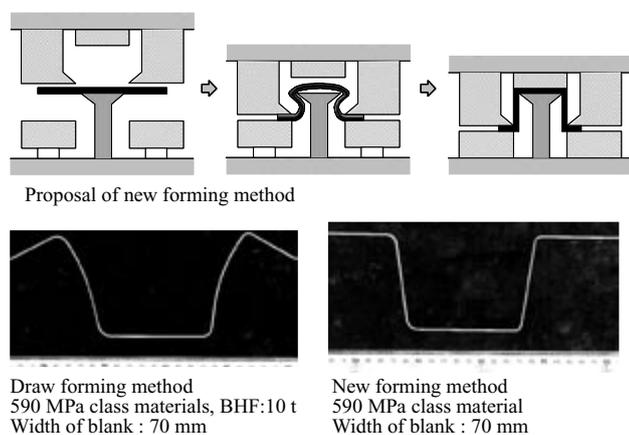
Fig. 16 Proposal of new forming method for improving shape fixability
