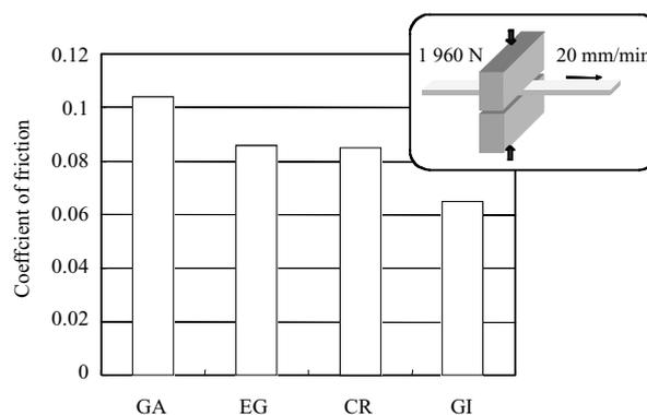
Fig.11 Influence of coating type on coefficient of friction
