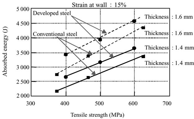
Fig. 17 Improving crashworthiness of hat square column by using new developed material
