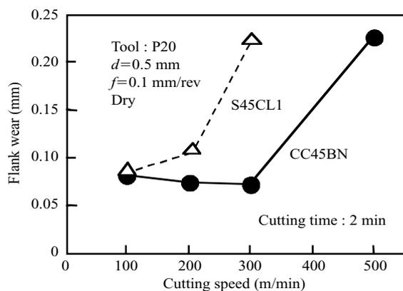
Fig. 28 Comparison of flank wear
